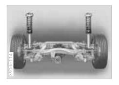
The illustration shows the rear axle of the sedan. With the lightweight, compact rear axle of the sport wagon, the shock absorbers are positioned at an angle.
