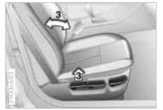
3 Backrest angle Pull the lever and apply weight to or remove weight from the backrest to reach the desired position
