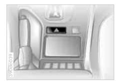
The button flashes rhythmically when the hazard warning flashers are on. To help you locate the switch in an emergency, the button is also illuminated whenever the car's headlamps are on.
