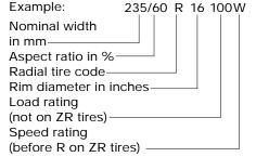
The speed rating indicates the approved maximum speed for the tire.
