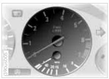
Indicates current fuel consumption in mpg (in liters per 100 km on Canadian vehicles). This instrument shows whether your current driving style is conducive to fuel economy with minimum exhaust emissions.
