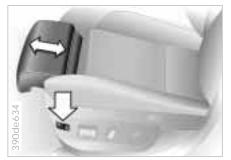
With this seat, you can also adjust the thigh support. To do that, press the switch.
