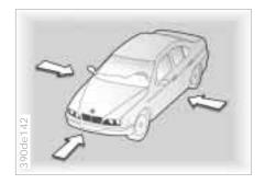
The illustration depicts schematically the primary directions of vehicle impact which initiate an airbag deployment.
