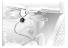
5 Then connect the negative terminals. Attach the cable to either the support vehicle's negative battery terminal, or to a suitable ground on its engine or bodywork. Then connect the other end of the cable to a ground on the engine or body of the vehicle which is to be started. There is a special nut on the strut dome of your BMW: refer to the arrow in the illustration.
