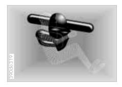
Deceleration sensors continuously monitor the physical forces acting upon the vehicle. If, as the result of a frontal collision, vehicle deceleration is reached at which the protection of the safety belts alone is no longer adequate, the gas generators of the driverside and passenger-side airbags are ignited simultaneously. However, the front airbag on the passenger-side is only triggered if an additional sensor has recognized that the passenger seat is occupied.
