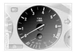
Never allow the engine to operate with the needle in the red overspeed zone of the gauge.
