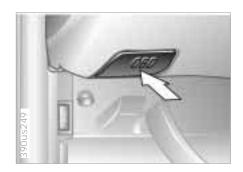
The Onboard Diagnostic (OBD) socket is located on the left of the driver's side at the bottom of the instrument panel and under a cover (arrow).
