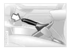
The parking brake is primarily designed to prevent the vehicle from rolling while parked. It operates against the rear wheels.
