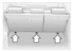
If you use a child restraint system with a tether strap, three additional tether anchorage points (refer to the arrows – the illustration shows the sport wagon) have been provided. Depending on the location selected for seating in the rear passenger area, attach the tether strap to the corresponding anchorage point to secure the child restraint system. Remove the cover first on the middle location.
