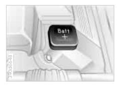
4 Start by connecting the jumper cable from the positive terminal of the support vehicle to the positive terminal connector located in your BMW's engine compartment. The cover of the auxiliary terminal for jump starting is marked with a "+" sign (refer to the illustration). Pull up to open the cover. The illustration shows the external positive terminal connector of the BMW 540i. For the BMW 525i, BMW 530i refer to "Engine compartment" on page 160.
