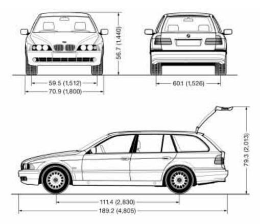
All dimensions are given in inches (mm). Height with roof-mounted luggage rack\*: 57.4 (1,459) Min. turning circle dia.: BMW 525i 37.1 ft (11.3 m), BMW 540i 37.4 ft (11.4 m)
